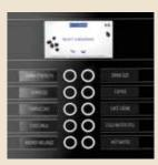
10 buttons Capacitive Keypad and a 4.3" Multicolour Display with RSS feed livens up the selection process by showing pictures and videos.
